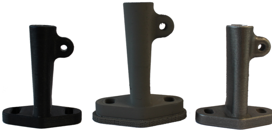
3D PRINTED PLASTIC PROTOTYPES (LEFT) ARE TESTED BEFORE METAL 3D PRINTING A GREEN PART (CENTER) AND SINTERING A FINAL DENSE METAL PART (RIGHT)
